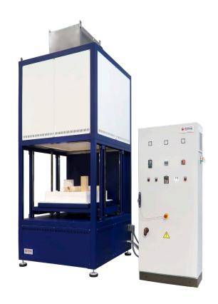
The bottom loading furnaces had the advantages of easy loading/unloading and tight sealing;
